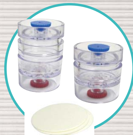
Preloaded 37-mm and 25-mm filters for hexavalent chromium sampling
