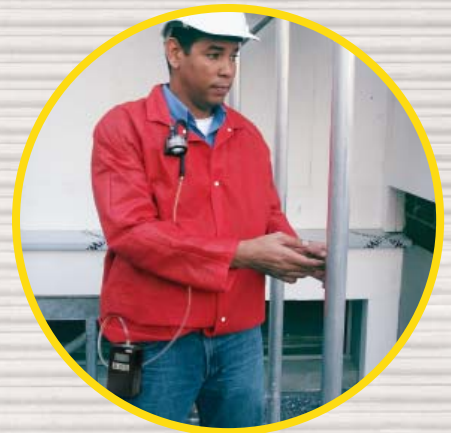
0.8- \mu\text{m} MCE filter and AirChek XR5000 sample pump for collecting lead in air
