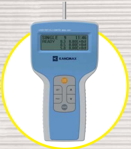
The handheld 3887 Optical Particle Counter for 3-channel measurement of particle sizes 0.3, 0.5, and 5.0 µm (3886 model measures 5 channels — 0.3, 0.5, 1.0, 3.0, and 5.0 µm)
